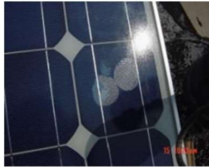
FIGURE 6. Partial shading of a PV module [7]
